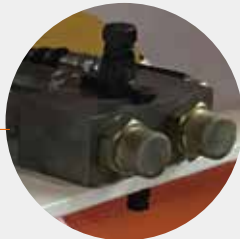
The control valve with output and input connector.
